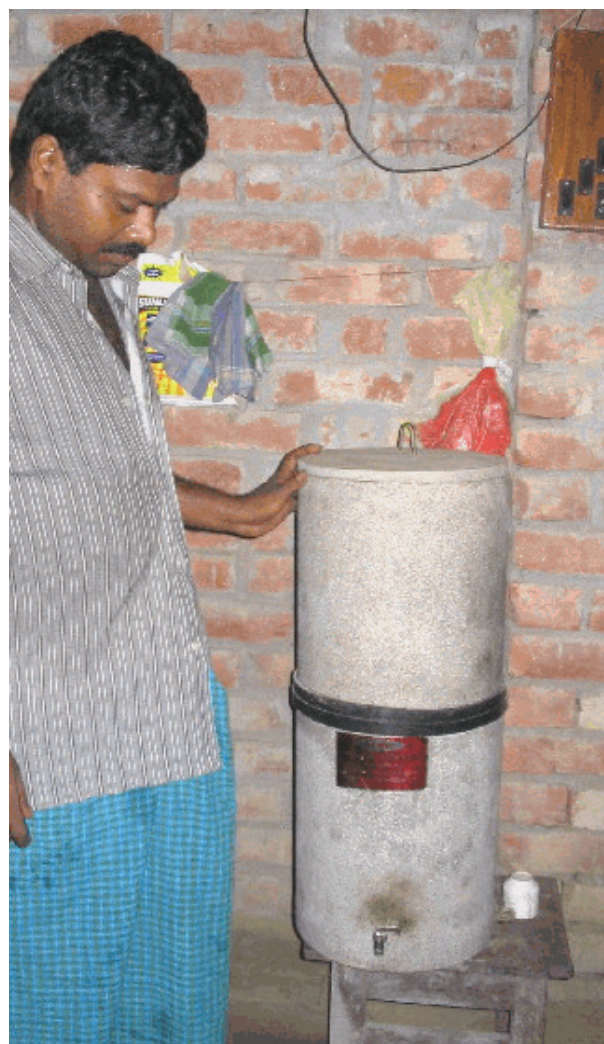
Picture 13: Nirmal combined arsenic and iron removal filter used in India
